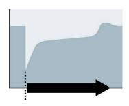
Sudden power demand from electric ignition followed by immeadiate power restoration from onboard alternator
