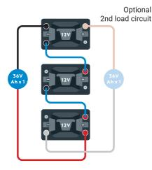
Basic principle illustrated other 'plus to plus' terminal connections can be used
